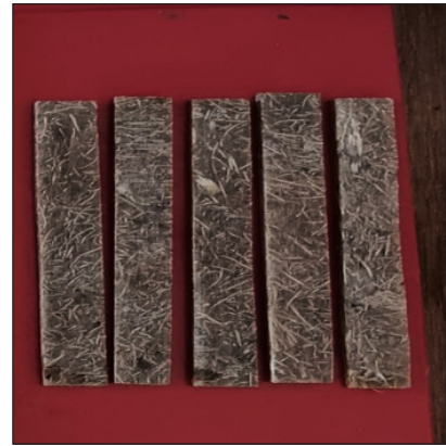
Figure 8. ISO 179 – Charpy impact test specimen (unnotched) Figure 9. Impact specimen
